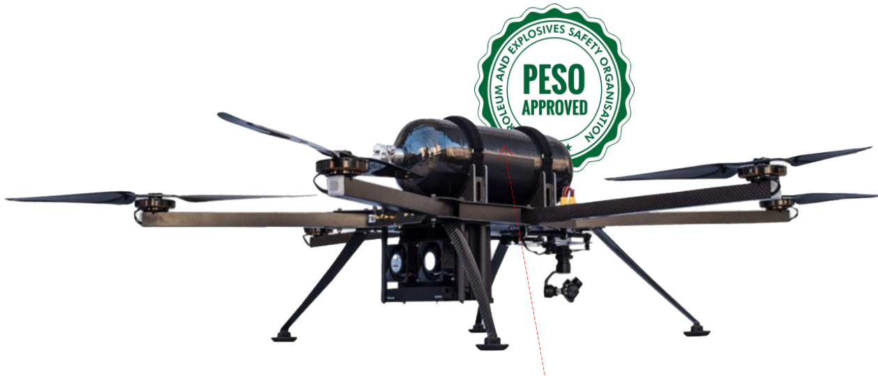
Hydrogen Type III Composite Cylinder
