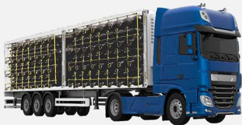
Type IV CNG Cylinder Cascades Lighter – Carries 220% More Gas
